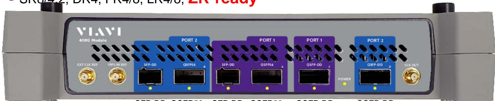
SFP-DD QSFP56 SFP-DD QSFP56 QSFP-DD QSFP-DD
